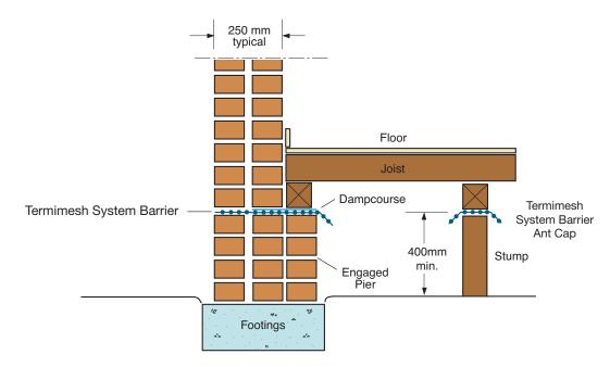
The Termimesh System Barrier is installed under the bearer. If the stump is timber or a brick pier, termites will be forced into the open to gain access.
