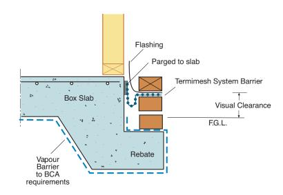
The Termimesh System Barrier is parged (bonded) to the side of the rebate, stepped down into the cavity and generally run on the second course of the outside brickwork below the flashing or dampcourse.
